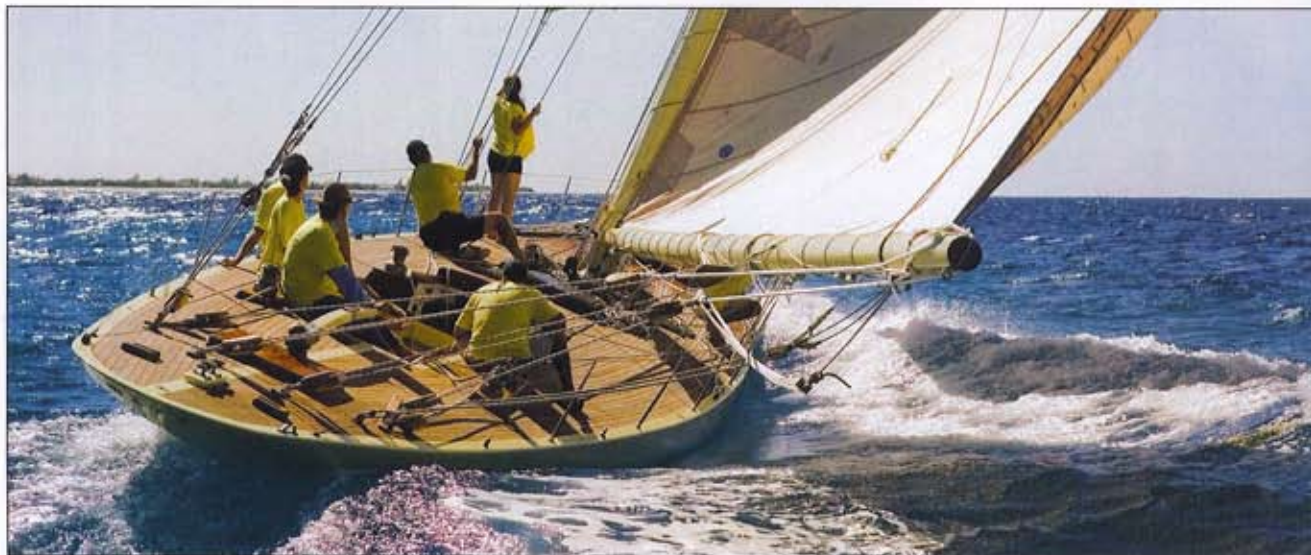
Some of KATE's deck hardware was obtained from TIGER, a 94' motoryacht that Philip Walwyn lost to sinking a year before the commencement of the 12-Meter's construction. The remainder of the hardware was cast in England. The spars are of Sitka spruce, milled in Alaska and shipped to St. Kitts. "I didn't calculate how much work was in the spars," says Walwyn. "It was 5-10 percent of the total job. That was a bit of a surprise."
