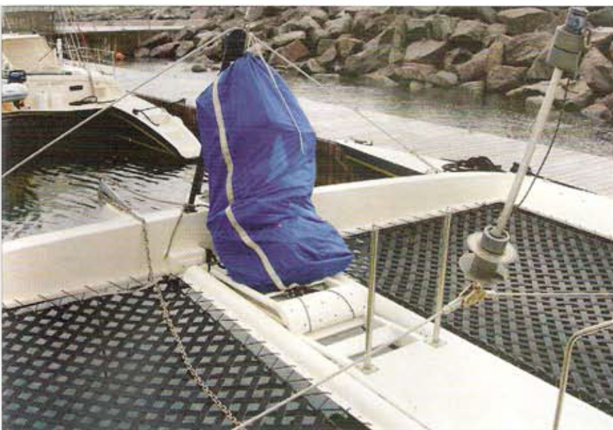
Protected by its blue bag, Eagle's boarding ladder deploys from between the trampolines on the foredeck, allowing passengers easy access when the cat is nudged onto a beach.
