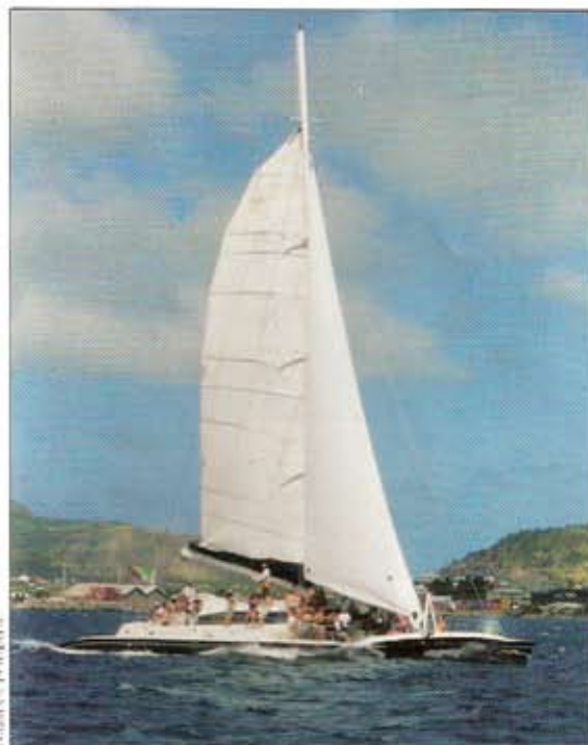
The 78' (23.7m) 14-ton Spirit of St. Kitts under way with a reefed main. Her hulls remain sound even after repairs brought about by extensive hurricane damage.
