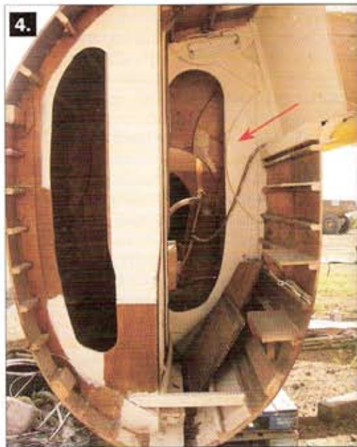
1 —Falcon's forward section shows some wear after 23 years of service. Note the elliptical box beam between bows, a Brookes departure from Spronk's square-shaped cross-members. 2 —Grinding scarfs into stringers. 3 —Brookes plans the keel scarf. 4 —A section view reveals the \frac{3}{8} "-Bruynzeel-plywood skin over Douglas-fir stringers on 6" (152mm) centers, and ring bulkheads every 4' (1.2m). The arrow points to a critical gusset in the structure.
