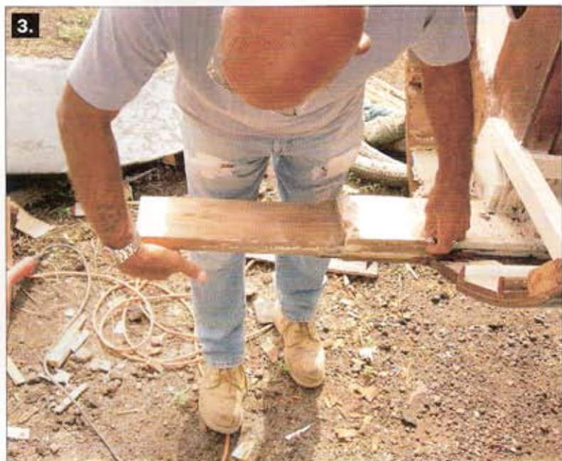
1 —Falcon's forward section shows some wear after 23 years of service. Note the elliptical box beam between bows, a Brookes departure from Spronk's square-shaped cross-members. 2 —Grinding scarfs into stringers. 3 —Brookes plans the keel scarf. 4 —A section view reveals the \frac{3}{8} "-Bruynzeel-plywood skin over Douglas-fir stringers on 6" (152mm) centers, and ring bulkheads every 4' (1.2m). The arrow points to a critical gusset in the structure.
